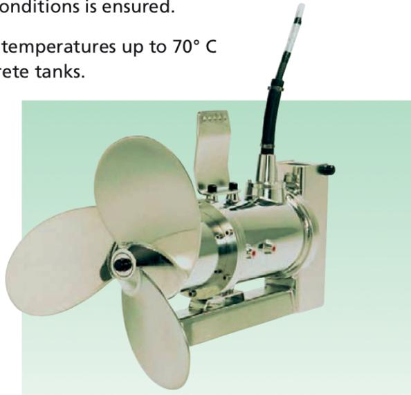
The Landia mixers have large-blade propellers with a low number of revolutions. Thus they are well suited and efficient for the mixing of sludge with a high dry matter content.
