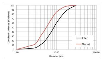
Fig. 3 - Particle size distribution used in simulation
